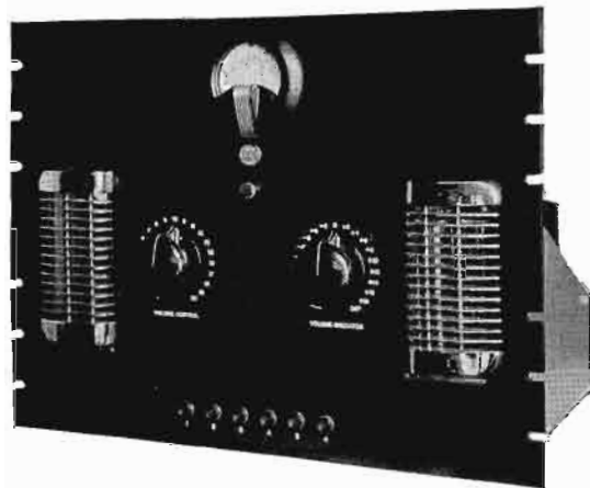
Front View of the DeLuxe 40-D Showing RCA's Modern Illuminated Meter Design Which Features Easy Bulb Replacement
